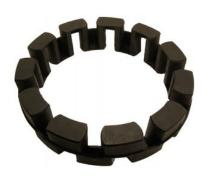
NM coupling consists of two hubs and flexible ring able to compensate all types of shaft misalignments. The flexible rings are made of Nitile rubber (NBR) which have a high internal damping characteristic which enable to absorb and dampen torsional vibrations, operate effectively in temperature range of -40 °C to +100 °C. The NBR material also resists to oil, dirt, grease, moisture, ozone and many chemical solvents.
